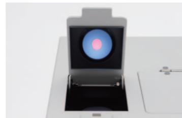
Opening the sample viewer provides a clear, illuminated view of the sample at the measurement port. On the CM-3600A, this view is reflected in a mirror so that you can view it easily even while seated.
